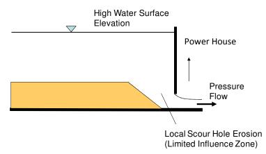
Figure 10: Pressure flushing to remove localized sediment deposits
